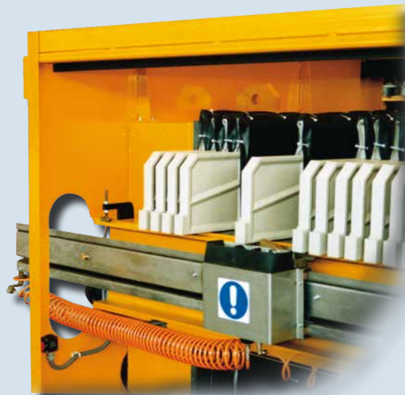
Exclusive automatic system filter plates translation and programmable shaking device
